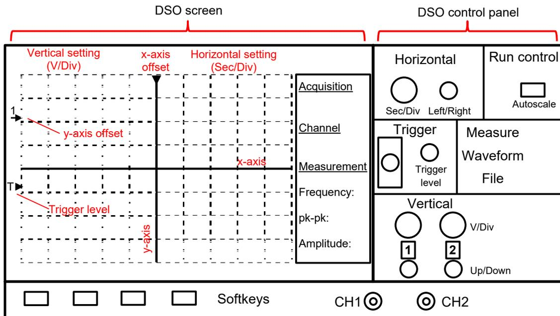
Fig. 4: DSO screen and control panel for DSO-X 2002A. For TDS 2014B, refer to the actual unit
