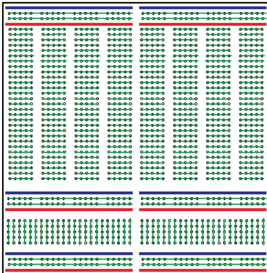
Fig. B: Breadboard picture and its internal connection
