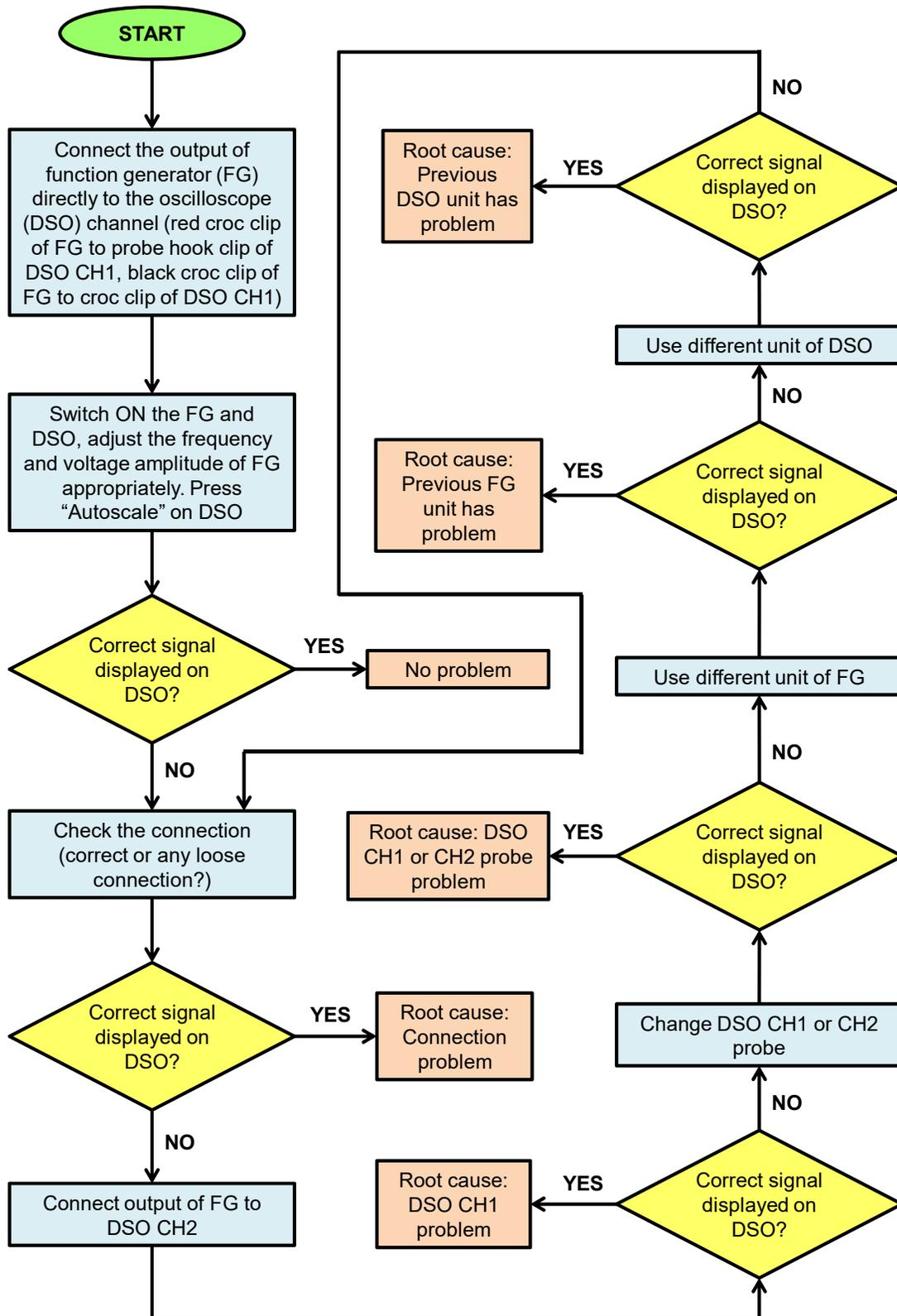
Fig. A: Flowchart of how to troubleshoot DSO and FG
